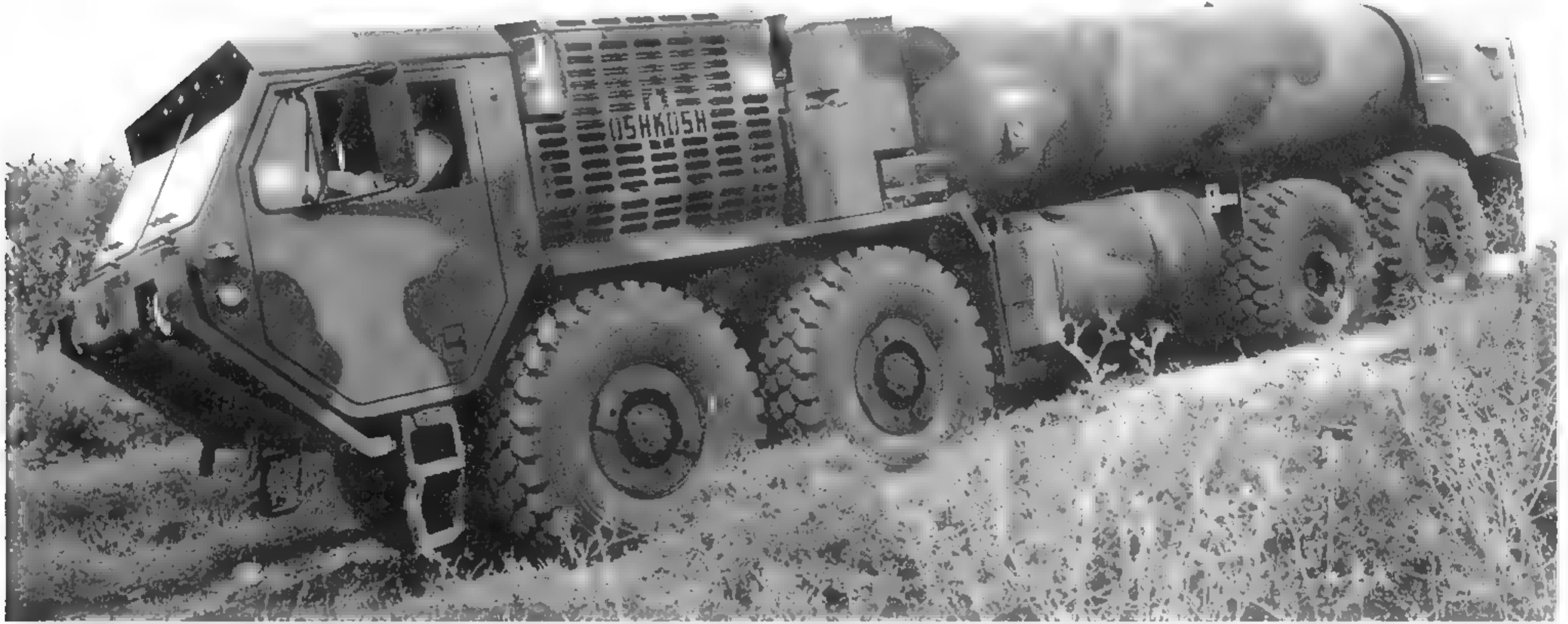
The M978 tanker has off-road mobility characteristics similar to those of the M977 cargo trucks. (U.S. Army photo)
